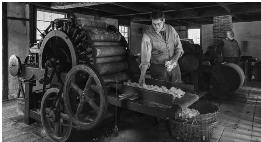
Carding is a mechanical process that disentangles, cleans, and intermixes fibers to produce a continuous web or sliver suitable for subsequent processing. This is achieved by passing the fibers between differentially moving surfaces covered with carding cloth. Photo courtesy of Old Sturbridge Village.
