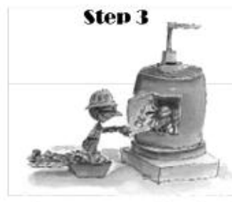
Step 3 The used cans go to the aluminum manufacturing plant. They are shredded, remelted with virgin aluminum and cast into new ingots.
