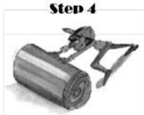
Step 4 The ingots are rolled into long, thin sheets that are then coiled and sent to the can manufacturing plant.
